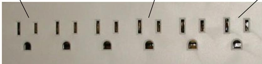
All the electrical plugs from the TV, VCR, Satellite Receiver, and any other device you want protected, should be plugged into the Surge Protector's outlet plugs.
