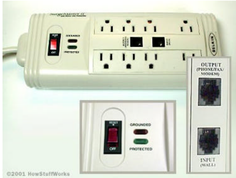
A Belkin SurgeMaster II mid-range surge protector with connections for phone lines
